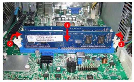
3. If a second memory module is available, install it in the DIMM2 slot by repeating step 1.
